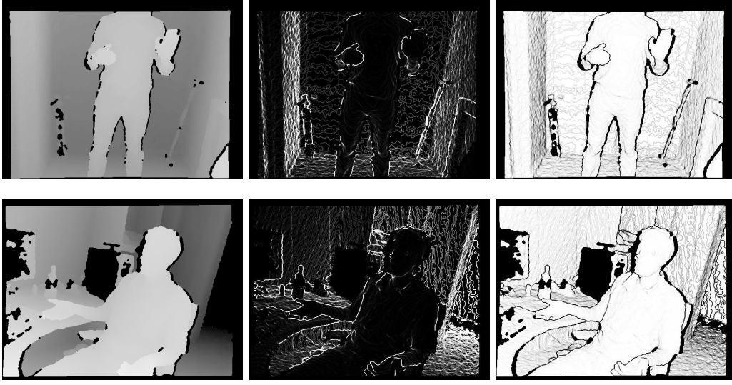
Fig. 5.5: Depth-based discontinuities preserving. From left to right: (a) depth image, Z(x) , (b) magnitude of the gradient, |\nabla Z(x)| , and (c) depth-based weighting function, c(\mathbf{x}) .
