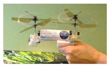
Figure 30 – The TwinCoAx micro aerial vehicle equipped with a single visual motion sensor looking downward which flew indoors over a natural scene. Reprinted from Ruffier and Expert (2012).
