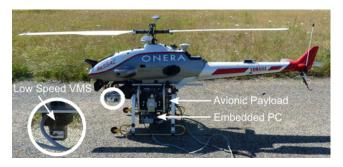
Fig. 6. The ONERA ReSSAC Unmanned Autonomous Helicopter before takeoff, featuring the on-board low-speed VMS mounted at the front end looking downward
