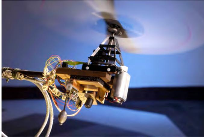
Figure 24 – The OCTAVE (Optic flow based Control system for Aerial VEHicles) robot is a 100g rotorcraft with 3 degrees of freedom (2 in position and 1 in attitude). Based on the optic flow regulation principle it is able to perform complex navigation tasks. Among these tasks we find taking-off, landing, wall following, and adjusting flight regime accordingly to wind disturbances. ©H. Raguet.
