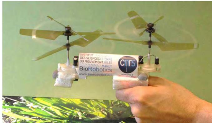
Figure 30 – The TwinCoAx micro aerial vehicle equipped with a single visual motion sensor looking downward which flew indoors over a natural scene. Reprinted from Ruffier and Expert (2012).
