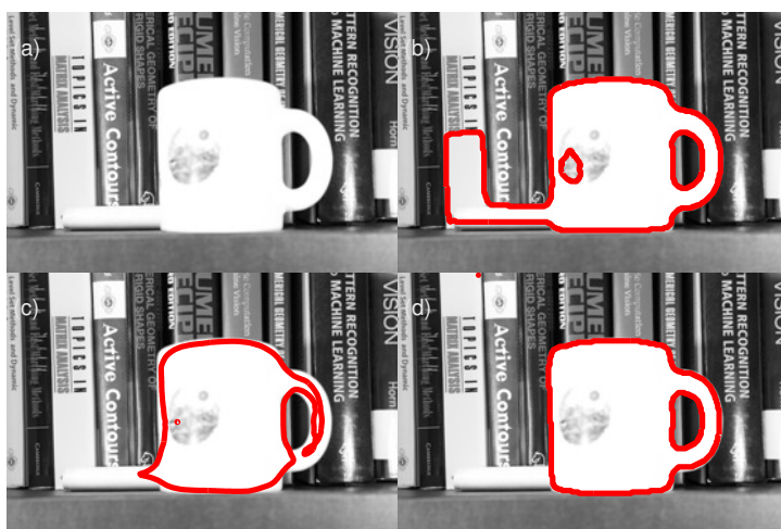
Figure 4.14: Segmentation results for the cup image (a) an image to be segmented, (b) result of segmentation using Chan-Vese model, (c) result of the segmentation using the multi-reference method from Foulonneau et al. , (d) result of the segmentation using the proposed method.
