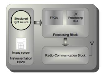
Figure 5.3: Block Diagram of the "Cyclope WCE"
