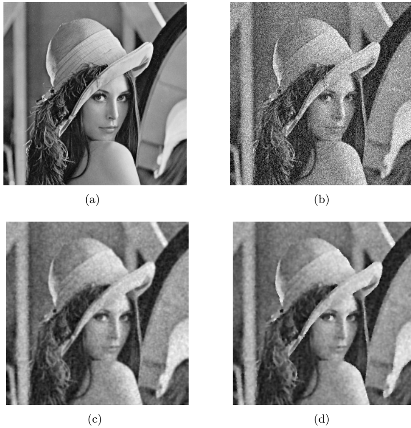
Figure 2.2: (a) Original image "lena" and (b) its corrupted version \psi_0 . Corrupting noise is a white Gaussian one of mean zero and standard deviation \sigma = 0.1 . (c) Restored image with usual Perona-Malik's approach, (d) Restored image with proposed approach.
