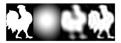
Figure 4.2: Images reconstructed from the Legendre moments with different orders. From left to right: original image and reconstruction images with orders  $N_o = 5, 20, 40$ .
