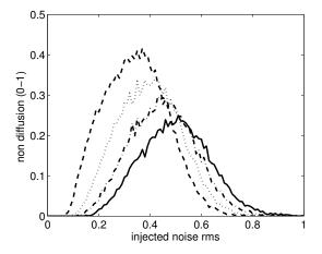
Figure 2.7: Ratio of non-diffused steps function of rms amplitude  $\sigma_{\eta}$ . N is fixed to 1000. Dashed line stands for k=0.65, dotted one for k=0.7, dash-dotted one for k=0.75 and solid one for k=0.8. For each value of k, the non-diffusion ratio is maximum for a non zero amount of purposely injected noise, which demonstrates the existence of a SR phenomenon.
