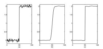
Figure 2.6: (a) Noisy step  $\psi_0$ , (b) Perona-Malik restoration of  $\psi_0$  (50 iterations), (c) Stochastic Perona-Malik restoration of  $\psi_0$  (50 iterations and  $\sigma_{\eta} = 0.3$ . Injection of  $\eta$  noise makes possible to obtain a better restoration of the noisy step regarding the fact that noise is suppressed and step discontinuity is preserved.
