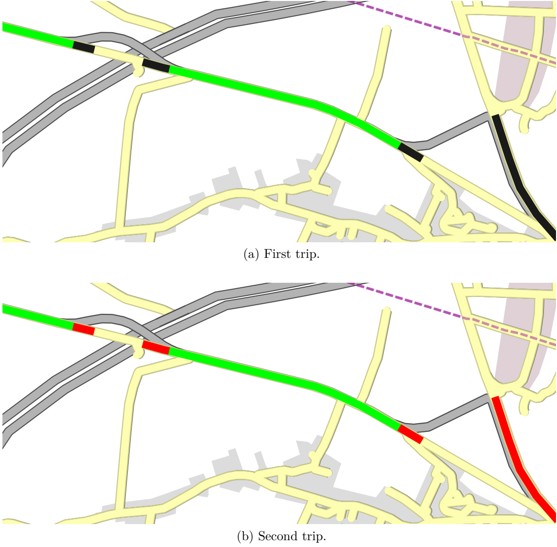
Figure 4.16: Results of the FDIA for the rural test track. The road sections for which the method states Use are in green, those for which the method states Don't use are in red and those for which the method states Unknown are in black. The true navigation map is in background in grey.
