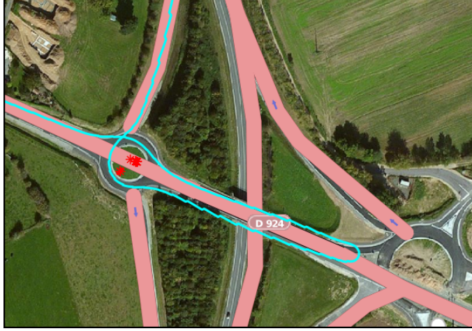
Figure 3.10: Example of application of the algorithm in rural environment. Here the road network has changed recently, one roundabout has been created and another one is being built. These are not registered in the navigation map (red lines) yet. The vehicle track is in blue and the centres of the roundabouts found by our algorithm are in red stars.
