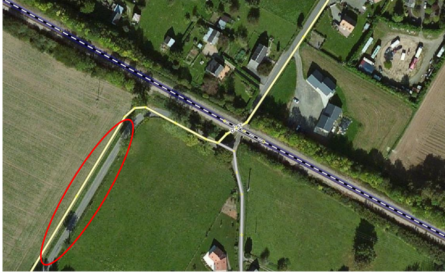
Figure 2.8: High confidence map-matching on a map fault. The road (circled in red) in the navigation map is 8 m aside the real road (assuming a perfect imagery). Since the road network is sparse, the confidence would be high despite this offset (OpenStreetMap data on top of Bing imagery).
