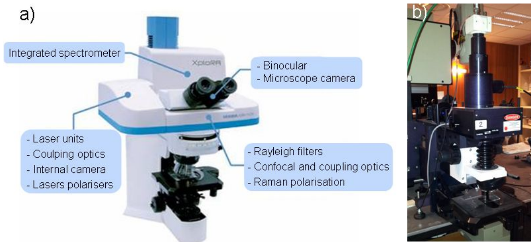
Figure 3.15: Micro-Raman spectrometers used in this work: a) Xplora-MV2000, b) T64000.
