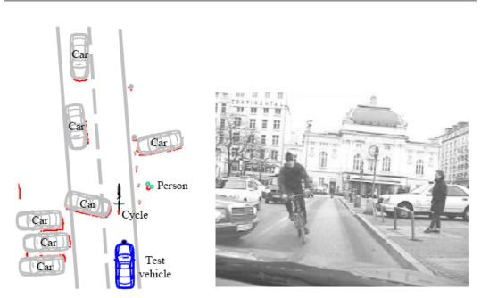
**Figure 1.3:** A goal of the vehicle perception with 2D lidar. Right: a real road scenario. Left: internal belief of the vehicle about it.
