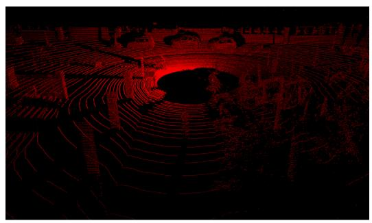
**Figure 1.4:** An illustration of the data provided by a single scan of Velodyne HDL-64E, a high definition lidar system for environment perception which consist of 64 laser beams rotating at 10Hz and covering a range of up to 120m.
