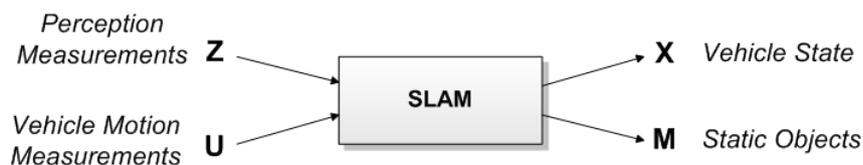
**Figure 2.1:** Simultaneous Localization and Mapping (SLAM).
