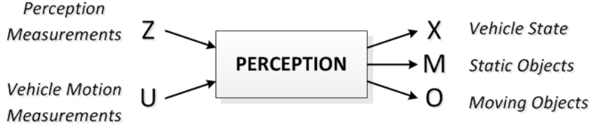
Figure 1.6: The general perception process. Z represents the perception measurements, U represents the motion measurements, X is the vehicle state, M is the map of stationary objects and O represents the states of moving objects.
