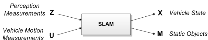
Figure 2.1: Simultaneous Localization and Mapping (SLAM).
