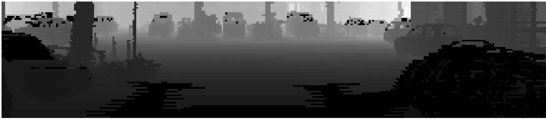
Figure 4.2: Sample of the Velodyne data stored in PNG distance image.
