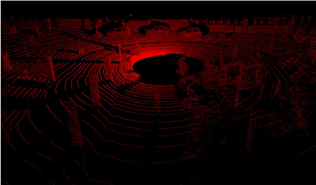
**Figure 1.4:** An illustration of the data provided by a single scan of Velodyne HDL-64E, a high definition lidar system for environment perception which consist of 64 laser beams rotating at 10Hz and covering a range of up to 120m.
