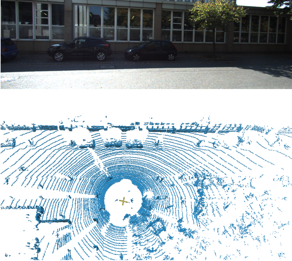
Figure 2.9: 3D Occupancy grid representation (bottom) of an outdoor scenario (top) that we will use to illustrate our approach for ground segmentation
