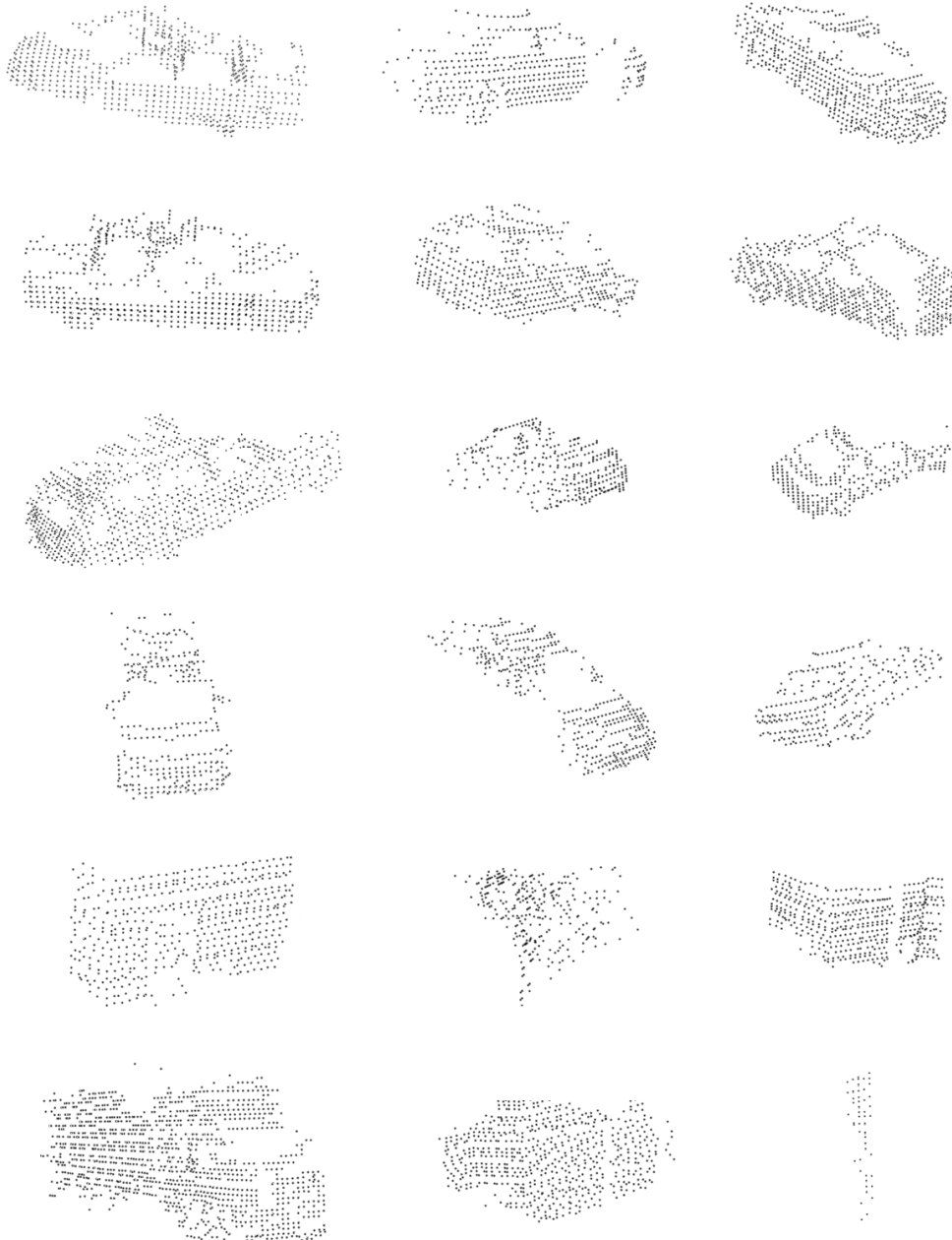
Figure 4.16: Some examples of the hand-labeled data used for training the car classifier. First four rows contain the positive examples while the last two rows contain the negative examples.
