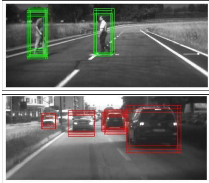
Figure 4.4: Output example from pedestrian (top) and vehicle classifiers (down) after being applied over the regions of interest from lidar moving object detection described in Section 4.1.1.
