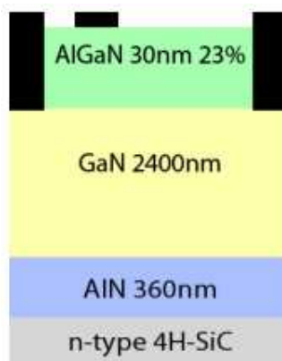
Figure 24 : Structure simple barrier
