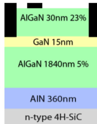
Figure 25 : structure double barriers
