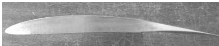
Figure 1.14: Turbine fan blade integrating an ABH extremity on the trailing edge (from [17])
