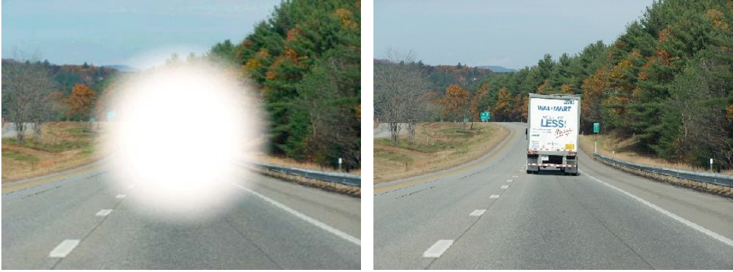
Figure 6.2: Delayed and undelayed operations. Frontal-blindness effect of delayed initialization ( left ) which leads to SLAM systems that only take into account fully observed landmarks, thus not those close to the motion axis. By considering also partially observed landmarks, an undelayed operation ( right ) is able to exploit all the available information.
