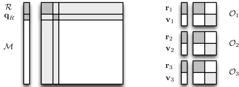
Figure 8.2: The SLAM-MOT map consists of the main BiCamSLAM map and a set of EKF, one per moving object.
