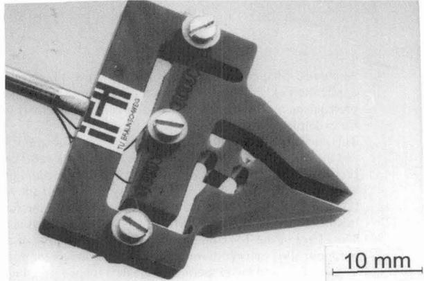
**Fig. 1:** Prototype of a miniature gripper for micro assembly using two helical springs in a differential actuator design [1].
