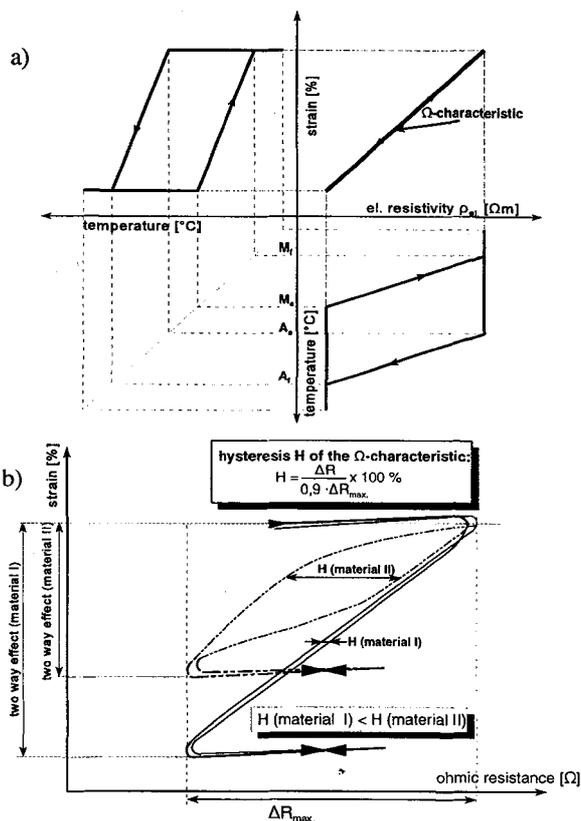
**Fig. 3:** Relationship between the electrical resistance and the shape change (strain) of a straight NiTi actuator wire (" $\Omega$ -characteristic curve"). The  $\Omega$ -characteristic is a superposition of two different relations, both of them showing a distinct hysteresis (a). Certain NiTi-based actuators offer this unique control property due to their small width of the resistance hysteresis (b).
