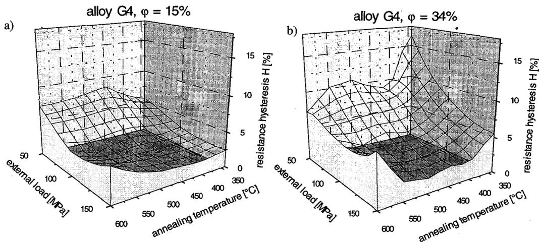
**Fig. 6:** Influence of the external load (a), of the amount of cold work (b) and of the annealing temperature on the  $\Omega$ -characteristic of alloy G4. Higher loads and intermediate annealing temperatures lead to decreasing amounts of H and therefore to better control properties.
