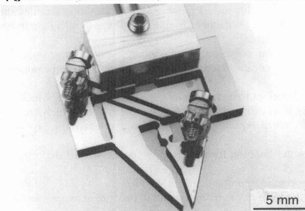
**Fig. 2:** Prototype of a miniature gripper for micro assembly using NiTiCu ribbon (alloy B25, **Tab. 1**) as an actuator and as a sensor simultaneously [1].
