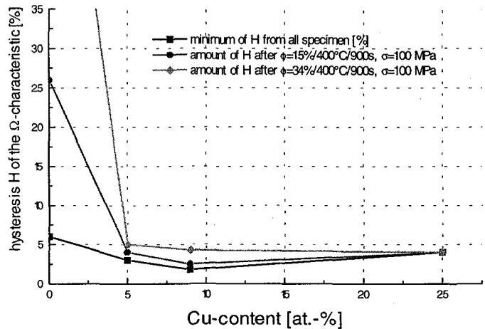
**Fig. 4:** Effect of the Cu-content and the cold work on the amount of hysteresis H in the  $\Omega$ -characteristic.
