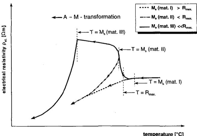
**Fig. 5:** The electrical resistivity of a binary NiTi alloy depends on the difference between the R and the M transformation temperatures. An increasing difference leads to a more pronounced anomaly of the specific resistivity [6].
