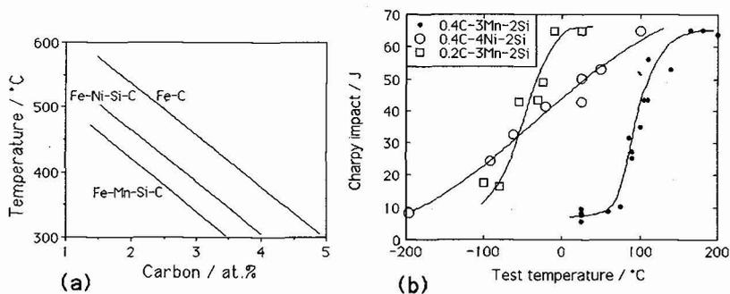
**Fig. 5:** (a) Calculated  $T'_0$  curves for the Fe-C, Fe-Mn-Si-C and Fe-Ni-Si-C steels. (b) Experimentally determined impact transition curves showing how the toughness improves as the amount of blocky austenite is reduced. The chemical compositions stated are approximate [15,16,17].
