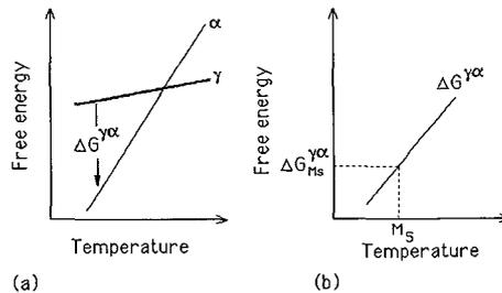
**Fig. 9:** (a) Difference in the free energies of austenite and martensite of the same chemical composition as a function of temperature. (b) Formation of martensite when the driving force achieves a critical value.
