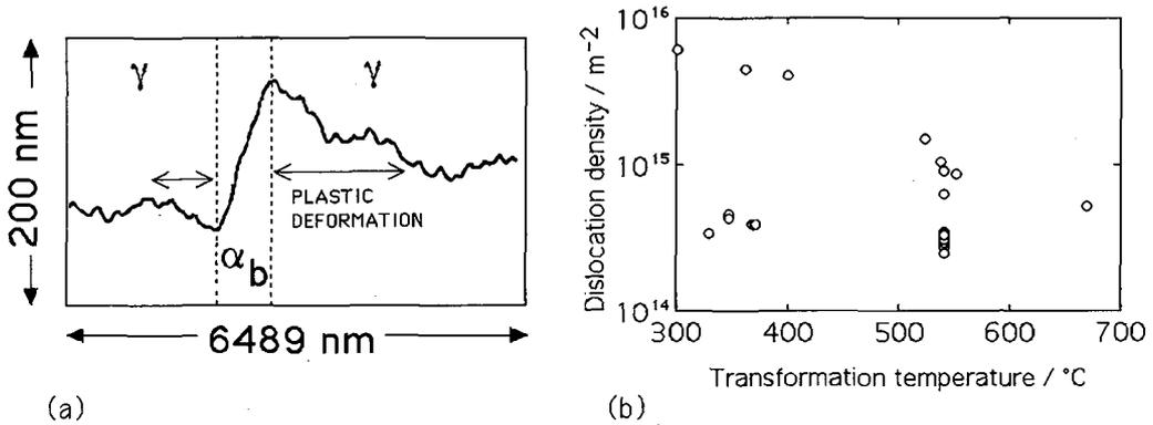
**Fig. 8:** (a) High-resolution atomic-force microscope plot of the displacements caused by the formation of a single sub-unit of bainite. The surface was flat before transformation. Note the plastic deformation caused in the adjacent austenite [24]. (b) Dislocation density of martensite, bainite and Widmanstätten ferrite as a function of the transformation temperature [32]
