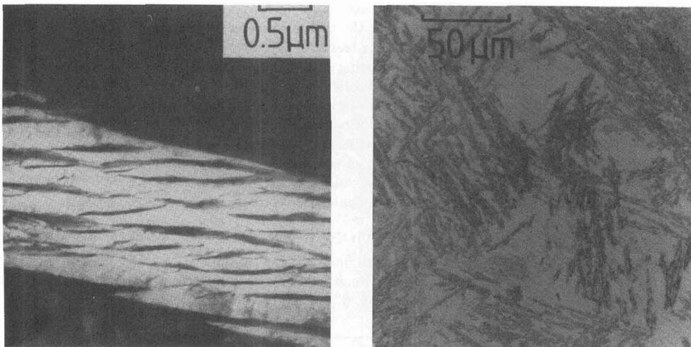
**Fig. 4:** (a) Transmission electron micrograph of a mixture of bainitic ferrite and stable austenite. (b) Optical micrograph of upper bainite in an Fe-0.43C-3Mn-2.02Si wt% showing the blocks of retained austenite between sheaves of bainite.
