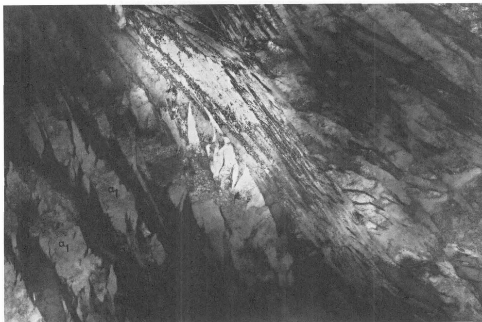
Figure 1: Bright field transmission electron micrograph of bainite obtained after isothermal treatment at 420°C for 30 min. and then at 290°C for 21 days. Two generations of bainitic ferrite and residual austenite are observed.
