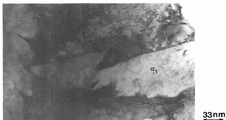
Figure 6: Bright field transmission electron micrograph of bainite obtained after isothermal treatment at 420°C for 30 min. and then at 290°C for 10 days. First generation of bainitic ferrite formed at 420°C (large needles) are observed embedded in austenite. High density of dislocations associated with the ferrite/austenite interface.
