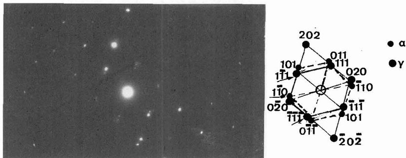
Figure 5: Selected Area Electron diffraction pattern corresponding to Fig.2 and its indexing. The orientation relationship between ferrite and austenite is close to the Kurdjumov-Sachs relationship.
