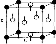
**Figure 1:** Representation of the tetragonal unit cell (fcc:  $c/a = 1.0$ , bcc:  $c/a = 1/\sqrt{2}$ ). Black and white circles mark (different) sorts of atoms. The spin order corresponds to a layered antiferromagnet.
