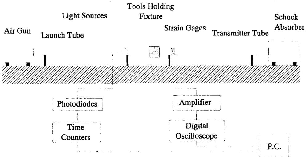
**Figure 1** : Schematic description of the experimental set up.
