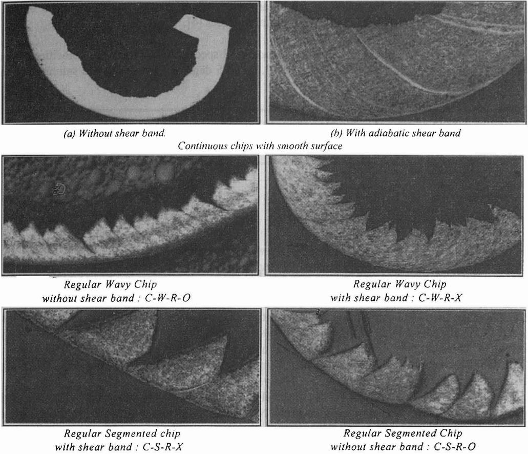
Figure 2 : Microscopic observations of different morphology of chips.
