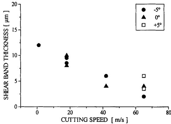
Figure 5 : Width of the Adiabatic Shear Band
