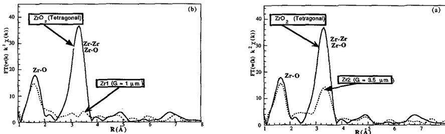
Fig 2: Fourier-transform magnitude spectrum (uncorrected for the phase shift) of standard (tetragonal-ZrO<sub>2</sub>) and polycrystalline doped- $\alpha$ -alumina samples: Zr2 (a) and Zr1 (b).
