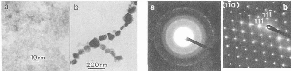
**Figure 1 :** Transmission electron microscopy images and diffraction patterns of the end products of the coprecipitation of  $\text{Fe}^{2+}$  and  $\text{Fe}^{3+}$  ions at  $\text{Fe}^{2+}/\text{Fe}^{3+} = 0.15$ , formed by a : process *i* ; b : process *ii* (see text) and separated by centrifuging.
