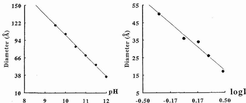
**Figure 2 :** Mean size of Fe<sub>3</sub>O<sub>4</sub> particles formed at different pH (I = 0.5 M) (left) and different ionic strengths (pH = 12) (right) after aging for 8 days at 25°C.
