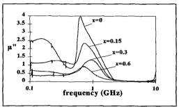
Figure 2 : imaginary part of the permeability in the unsaturated state on  $Y_{1-x}Dy_xGd_2Fe_5O_{12}$  polycrystalline toroïds.
