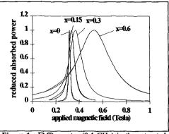
Figure 1 : FMR spectra (9.4 GHz) in the saturated state on  $Y_{1,x}Dy_xGd_2Fe_5O_{12}$  single crystal spheres.
