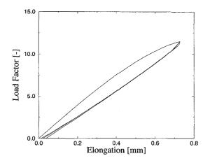
Figure 1. Load versus end displacement of the bar for three different discretisations.
