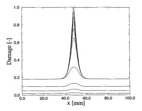
Figure 2. Damage evolution along the bar for progressive loading.
