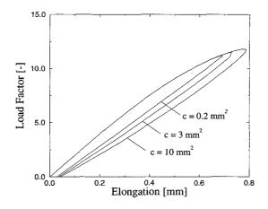
Figure 4. Load versus end displacement of the bar for different values of the gradient parameter.
