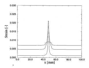
Figure 3. Strain evolution along the bar for progressive loading.
