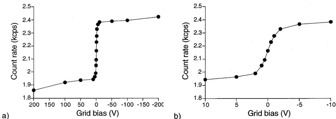
**Figure 2.** Plot of the ion rate as a function of grid voltage: (a) over the range +200 to -200 V grid voltage and (b) over the range +10 to -10 V. Note that the noise level during these measurements was approximately 100cps, and has not been subtracted from the data shown in the graphs.
