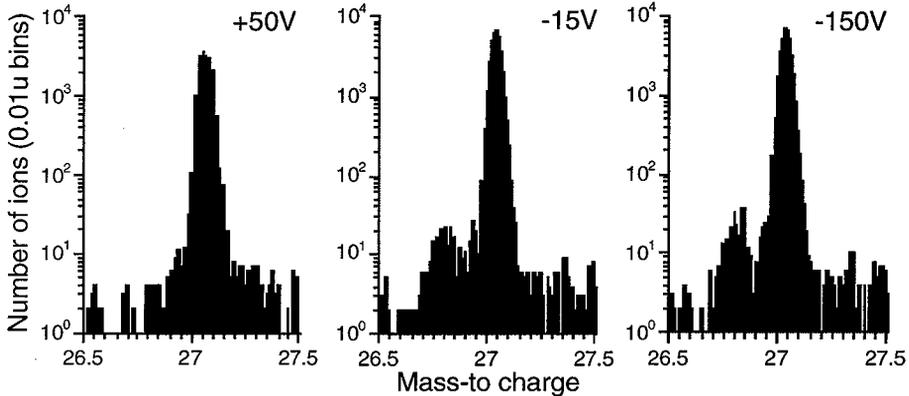
**Figure 3:** Comparison of mass spectra for  $\text{Al}^{2+}$  ions in the energy compensated optical PoSAP system, for different grid bias. The grid potentials given in each case are quoted with respect to the front face of the MCP, which was set to -50V.
