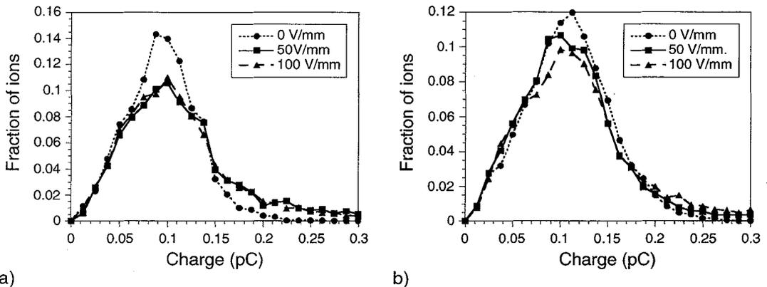
**Figure 6:** Pulse height distributions from the work of Deconihout *et al.*, [4]: (a) from the area of the MCP covered by the grid; (b) from the uncovered area of the MCP.
