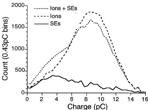
**Figure 1:** Pulse height distributions from the OPOsAP detector with the grid over the detector biased to +200V (PHD due to ions alone) and -200V (distribution from both ions and secondary electrons). By subtracting the first distribution (suitably scaled) from the second, the distribution due to the secondary electrons (SEs) is obtained.
