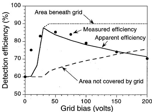
**Figure 5:** Variation in efficiency over different regions of the test detector used by Deconihout *et al.* and the overall efficiency which would have been measured by comparing the two and assuming an open area of 60%. The efficiency data from Deconihout *et al.* are shown for reference (points).
