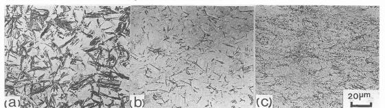
Fig. 4 Optical metallographs showing the microstructures obtained from the dilatometric specimens isothermally treated at 370°C for 30 min with different amounts of prior deformation: (a) 0%, (b)10% and (c) 40%.
