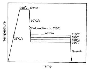
Fig. 1 Schematic diagram showing the main thermo-mechanical processes performed in the dilatometer.
