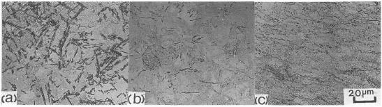
Fig. 2 Optical metallographs showing the microstructures obtained from the dilatometric specimens isothermally treated at 410°C for 30 min with different amounts of prior deformation: (a) 0%, (b)10% and (c) 40%.
