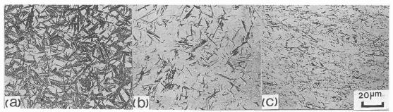
Fig. 5 Optical metallographs showing the microstructures obtained from the dilatometric specimens isothermally treated at 350°C for 30 min with different amounts of prior deformation: (a) 0%, (b)10% and (c) 40%.
