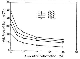
Fig. 8 Plot of the volume fraction of bainite versus the amount of prior deformation for different isothermal temperatures. The volume fractions of bainite were obtained after the reactions of bainite had been complete.
