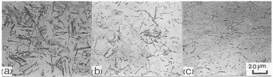
Fig. 3 Optical metallographs showing the microstructures obtained from the dilatometric specimens isothermally treated at  $390^{\circ}$ C for 30 min with different amounts of prior deformation: (a) 0%, (b) 10% and (c) 40%.
