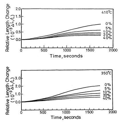
Fig. 7 Dilatometric curves for isothermal transformation at (a) 410°C and (b) 350°C with and without prior deformation (the amounts of prior deformation indicated).
