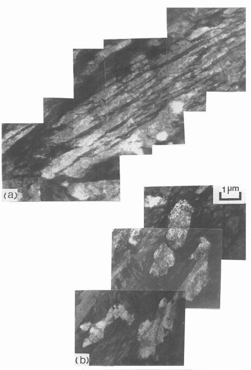
Fig. 6 Transmission electron micrographs (a) and (b) showing the microstructures for corresponding optical metallographs of Figs. 5(a) and 5(c) respectively.
