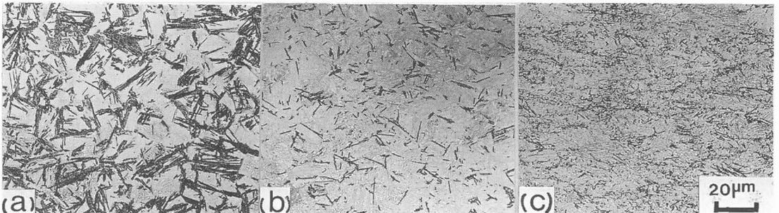
**Fig. 4** Optical metallographs showing the microstructures obtained from the dilatometric specimens isothermally treated at 370°C for 30 min with different amounts of prior deformation: (a) 0%, (b) 10% and (c) 40%.
