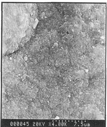
Figure 9 : AlN and \text{Si}_3\text{N}_4 codeposit. Deposition conditions: T = 1200\text{ }^{\circ}\text{C} , P = 1\text{ Torr} , T_c = 416\text{ }^{\circ}\text{C} .
