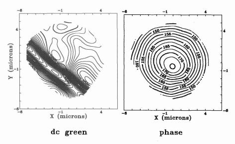
Figure 1: Green reflectance map (left) and phase map (right) obtained on a sample of bulk gold (modulation frequency: 1 MHz). A surface scratch clearly appears on the reflectance map, but does not perturb the phase of the photothermal signal.
