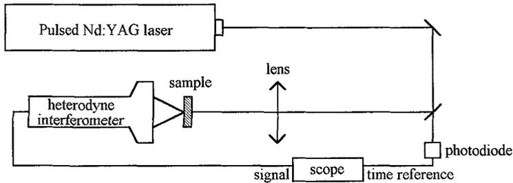
Figure 3: scheme of the laser-ultrasonics experiment
