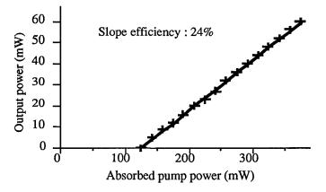
Figure 4 : slope efficiency in <u>pure cw</u> with the 3 % doped crystal
