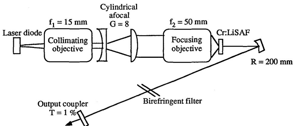
Figure 1 : experimental set-up.
