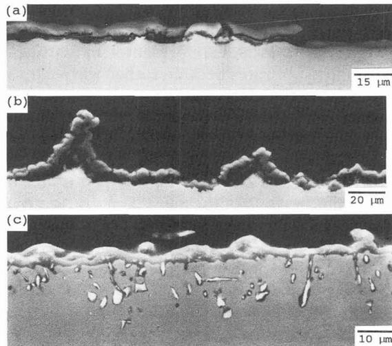
Fig. 3. — Polished cross-sections of Al<sub>2</sub>O<sub>3</sub> formed at 1100 °C for 50 hours on: a) untreated Fe-18Cr-5Al; b) La-implanted Fe-18Cr-5Al; c) La-implanted Fe-18Cr-5Al-1Hf.
