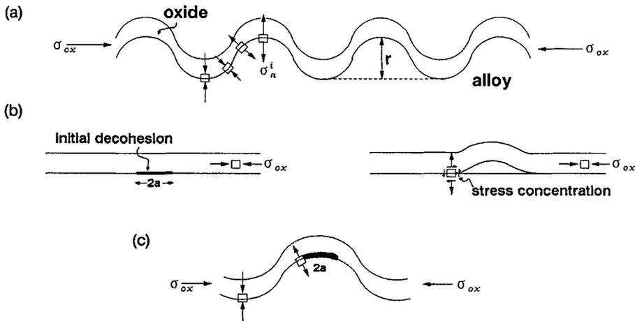
Fig. 8. — Schematic illustrations of a) the wavy interface developed on the La-implanted Fe-Cr-Al alloy and the local stress concentration at asperities; and the effect of scale decohesion on crack extension on: b) a flat interface; c) a wavy interface.
