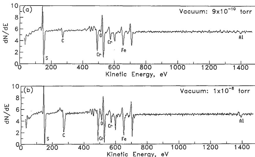
Fig. 7. — Typical Auger analyses of the substrate surface on: a) untreated Fe-Cr-Al alloy; b) La-implanted Fe-Cr-Al, after removal of the surface scales under ultra high vacuum. The surface scales were formed at 1100 °C for 15 minutes in oxygen.
