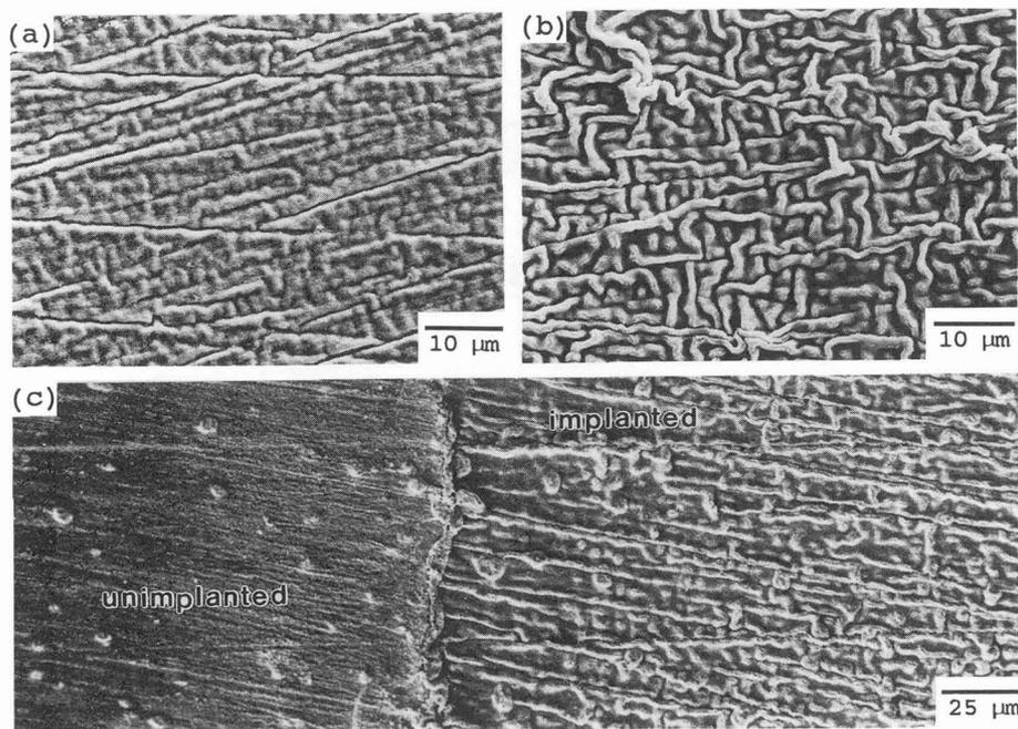
Fig. 1. — Morphology of  $\text{Al}_2\text{O}_3$  scales formed after 15 minutes at  $1100^\circ\text{C}$  on: a) untreated Fe-18Cr-5Al; b) La-implanted Fe-18Cr-5Al; c) La-implanted Fe-18Cr-5Al-1Hf near the implanted/unimplanted interface region.
