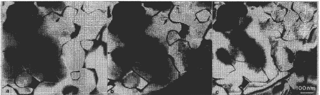
Figure 7: Comparative DF images showing the microstructure of the APB in \text{Co}_{37}\text{Pt}_{63} ordered with the \text{L}_{12} structure: (110) in a), (210) in b), (120) in c). The APB which should be out of contrast in a given dark field appears with a white contrast because of the wetting by \text{L}_{10} .
