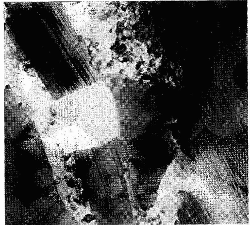
Fig. 5 Transmission electron micrograph of an Al-6wt.%Fe + 10 vol.% SiC particle powder extrusion. \square 1 \mu m
