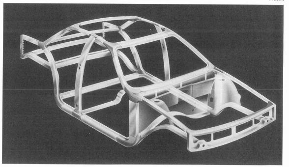
This Rendering of a Generic Spaceframe Illustrates the Use of Less than 100 Aluminum Extrusions and Interconnecting Aluminum Die Cast Nodes which are Robotically Welded to Form the Car Body. A Limited Number of Aluminum Sheet Components (i.e. Inner Fenders, Floor Pan) are then Attached to Complete the Body.
