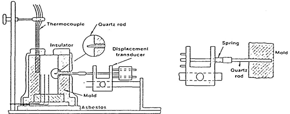
Figure 1. Solidification test: schematic of the experimental setup of Nishida et al. [6].
