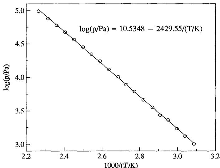
Fig. 2. — Vapour pressure of tetraethoxysilane from 323 to 441 K.
