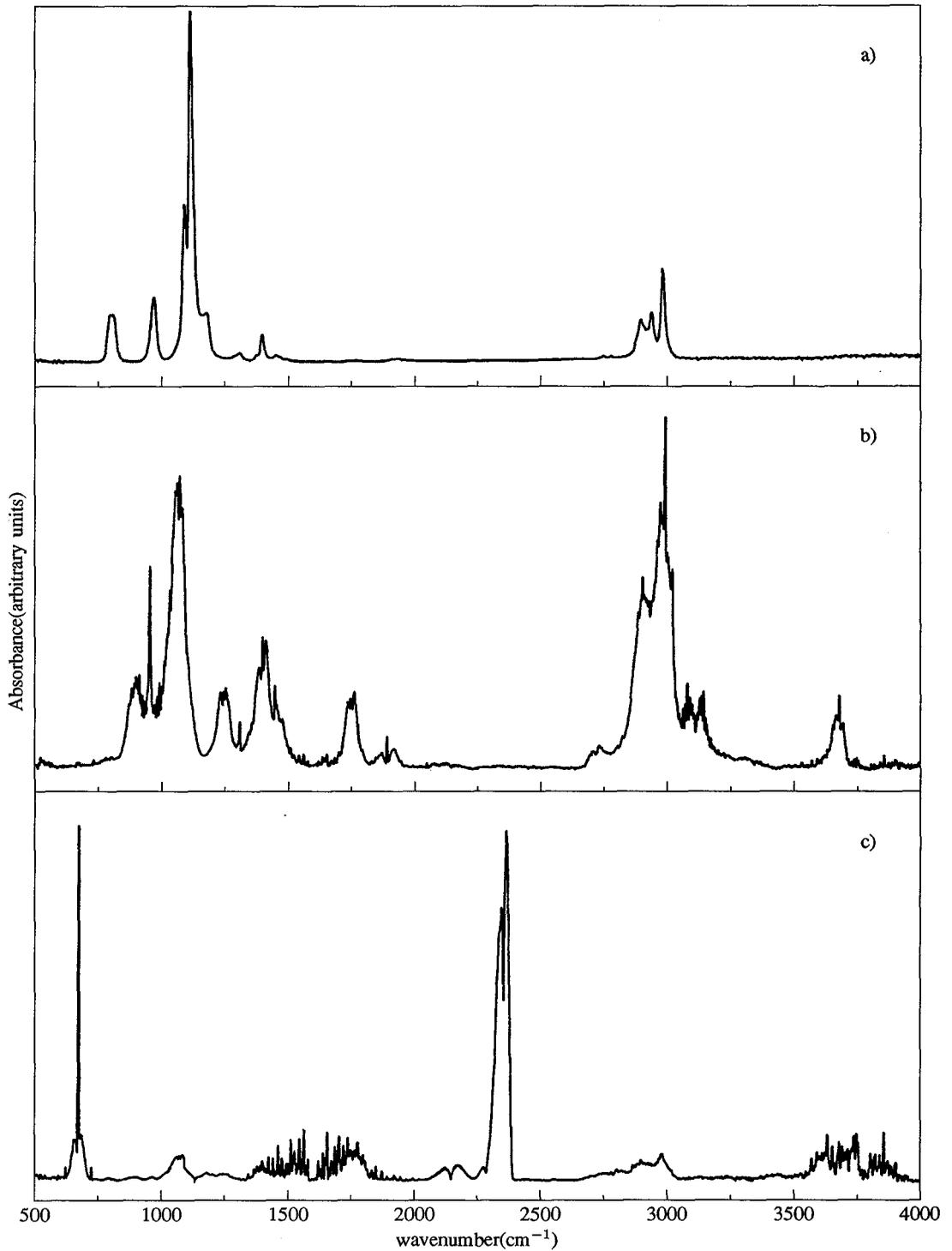
Fig. 3. — Infrared spectra of a) TEOS, b) product spectrum of pyrolysis at low pressure, and c) product spectrum of pyrolysis at atmospheric pressure in oxygen.
