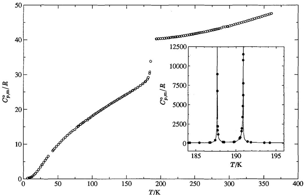
Fig. 1. — Low-temperature heat capacity of tetraethoxysilane.
