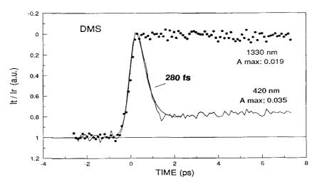
Figure 3 : Typical normalized kinetics of induced absorption vs time in neat DMS at 294 K for two test wavelengths (420 and 1330 nm) following femtosecond ultraviolet excitation. The maximum of absorbance at 420 nm is about twice that value obtained at 1330 nm. The absorbance at long time is due at least partially to the formation of the secondary anion  $CH_3SSCH_3$ . At 420 nm, the transient species exhibits a lifetime of  $280 \pm 10$  fs
