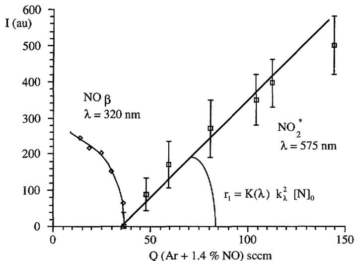
Fig. 2. — N-atom titration plot for an Ar-4% N<sub>2</sub> afterglow at  $P = 300$  Pa,  $Q = 520$  sccm and  $W = 130$  W.
