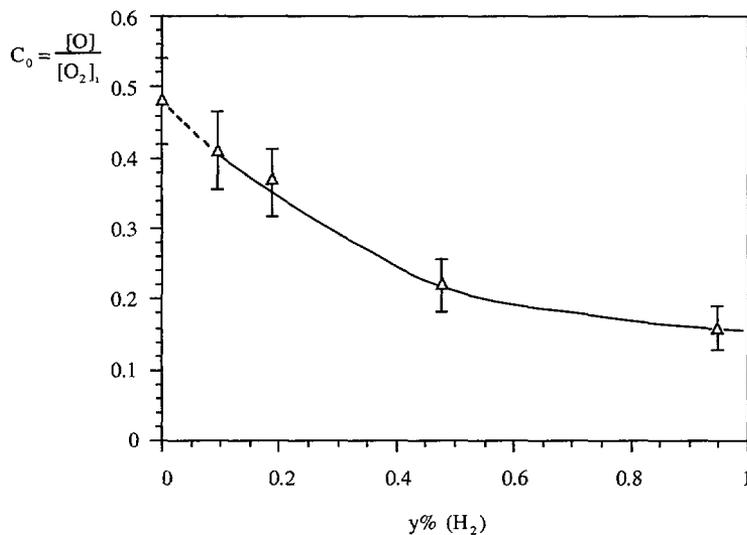
Fig. 5. — Relative O-atom density ( $C_0$ ) versus hydrogen percentage ( $y\%$ ) for an Ar-1.2%  $O_2$ - $y\%$   $H_2$  microwave discharge at  $P = 1\,500 \text{ Pa}$ ,  $1\,039.5 \leq Q \leq 1\,049.5 \text{ sccm}$  and  $W = 130 \text{ W}$ .
