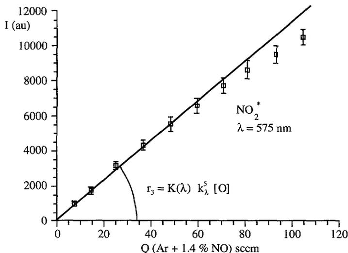
Fig. 4. — O-atom titration plot for an Ar-3.8%  $O_2$ -0.2%  $H_2$  afterglow at  $P = 300 \text{ Pa}$ ,  $Q = 521 \text{ sccm}$  and  $W = 130 \text{ W}$ .
