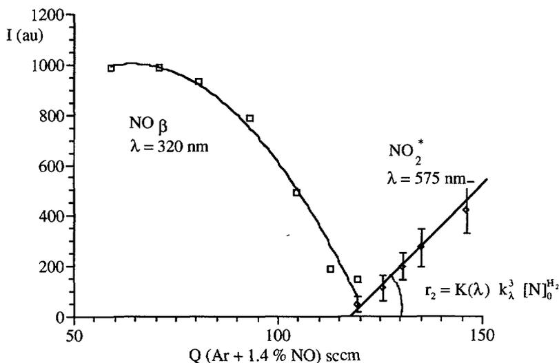
Fig. 3. — N-atom titration plot for an Ar-3.8% N<sub>2</sub>-0.2% H<sub>2</sub> afterglow at  $P = 300$  Pa,  $Q = 521$  sccm and  $W = 130$  W.
