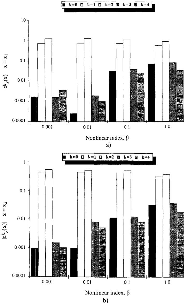
Fig. 2. — Amplitudes of the harmonic components of the electric field *versus* the nonlinear parameter  $\beta$ , for  $\epsilon_b = 4.0$ , inside the dielectric object (Fig. 1) at the positions a)  $\mathbf{x}_1 = (0,0,0)$ , b)  $\mathbf{x}_2 = (\lambda_0/100, 0, 0)$ , c)  $\mathbf{x}_3 = (0, \lambda_0/100, 0)$ , d)  $\mathbf{x}_4 = (-\lambda_0/100, 0, 0)$  and e)  $\mathbf{x}_5 = (0, -\lambda_0/100, 0)$ .
