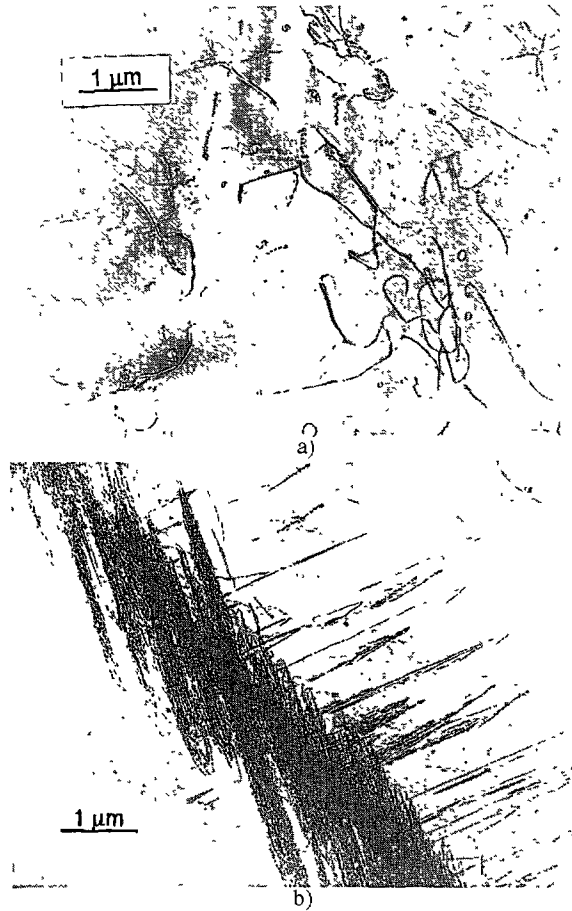
Fig. 8. — a) Dislocation microstructure typical of recovery in a crystal with [H]/[Si] \approx 180 at. ppm. Compression axis // O^+ . T = 700 °C, P = 1000 MPa, \dot{\epsilon} = 10^{-6} s^{-1} b) Dislocation microstructure typical of a Peierls regime in a wet quartz with [H]/[Si] \approx 100 at. ppm. Deformation conditions identical to a).
