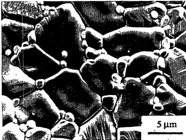
Fig. 5. — Precipitation of yttrium garnet in yttrium doped alpha alumina polycrystals [18].
