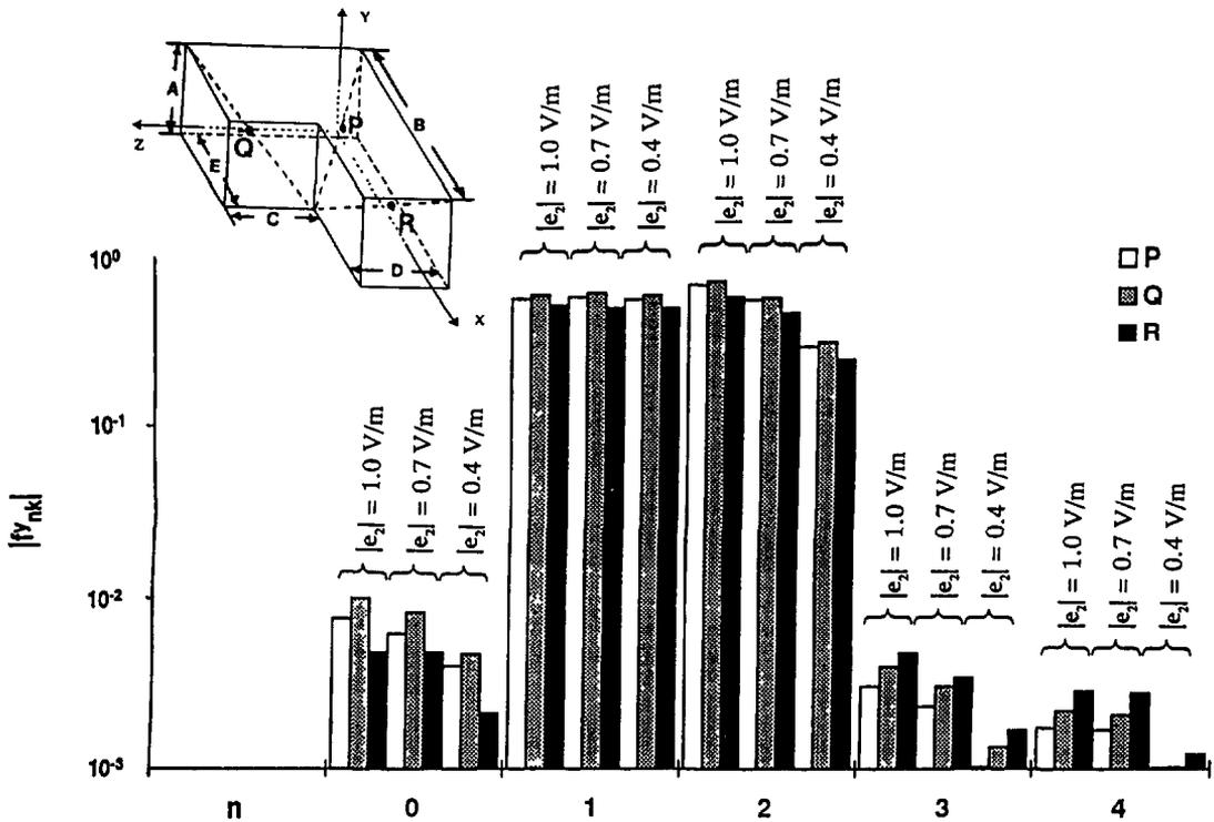
Fig. 6. — Nonlinear scatterer ( $A = 1/2 B = C = D = E = \lambda / 30$ ) and coefficients  $|f_{nk}^y|$  for different values of  $|e_2|$ . In this case :  $\eta = 0.01$ ,  $\epsilon'_t = 2.0$ ,  $N = 4$ ,  $X = 25$ .
