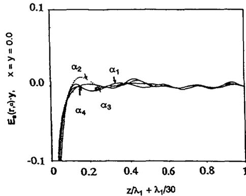
Fig. 7. — External scattered electric field ( $y$ -component) along the propagation axis ( $z$ -axis), for  $\eta = 0.1$ ,  $\varepsilon'_r = 2.0$ ,  $N = 6$ ,  $X = 40$ ,  $\alpha_i = (i - 1)/5 \nu_1$ .
