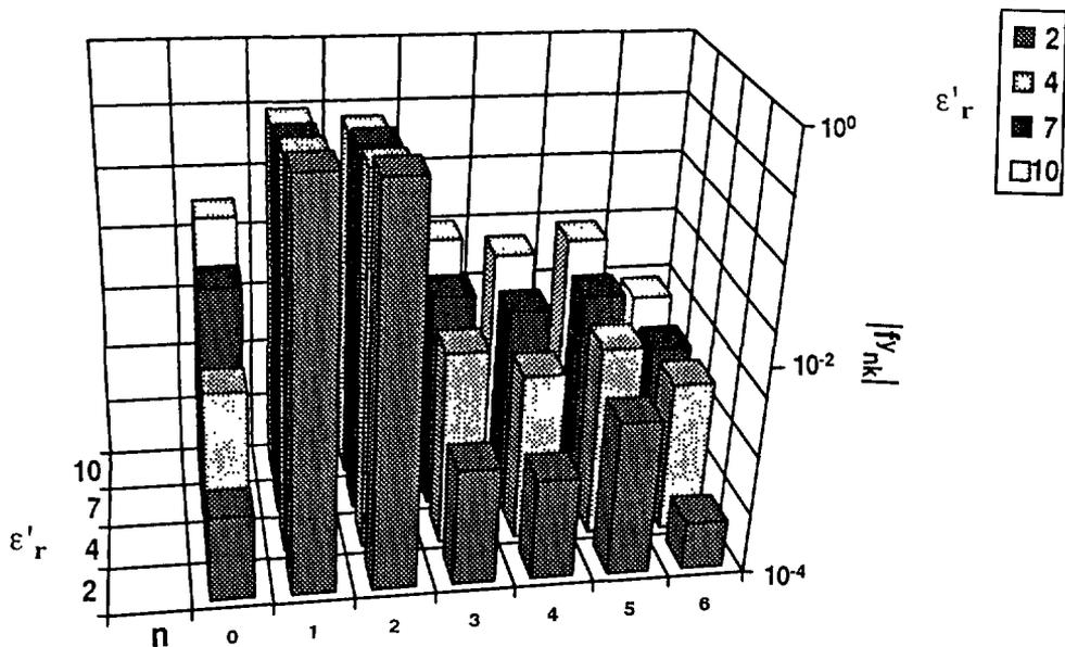
Fig. 3. — Coefficients  $|f'_{nk}|$  *versus* the linear part of the dielectric permittivity  $\epsilon'_r$ , for  $\eta = 0.1$ ,  $N = 6$ ,  $X = 40$ .
