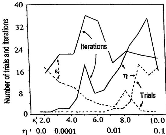
Fig. 2. — Numbers of trials and iterations *versus* the  $\eta$  values, for  $\epsilon'_r = 2.0$ ,  $N = 6$ ,  $X = 40$ , and *versus* the  $\epsilon'_r$  values, for  $\eta = 0.1$ ,  $N = 6$ ,  $X = 40$ .
