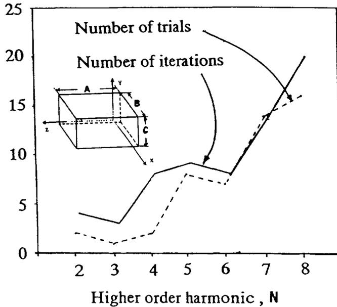
Fig. 4. — Numbers of trials and iterations for different values of  $N$  (highest-order harmonic component). In this case :  $\eta = 0.01$ ,  $\epsilon'_r = 2.0$ ,  $N = 5$ ,  $X = 25$  ( $A = 2 B = 2 C = \lambda / 15$ ).
