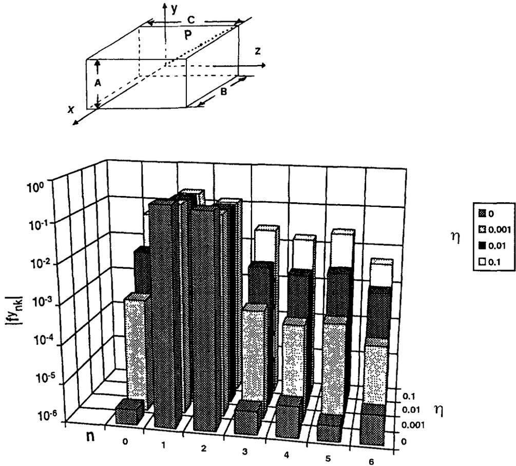
Fig. 1. — Nonlinear dielectric parallelepiped ( $A = 1/2 B = 1/2 C = \lambda_1/30$ ) and coefficients  $|f_{nk}^y|$  versus the nonlinear parameter  $\eta$ , for  $\epsilon'_r = 2.0$ ,  $N = 6$ ;  $X = 40$ .
