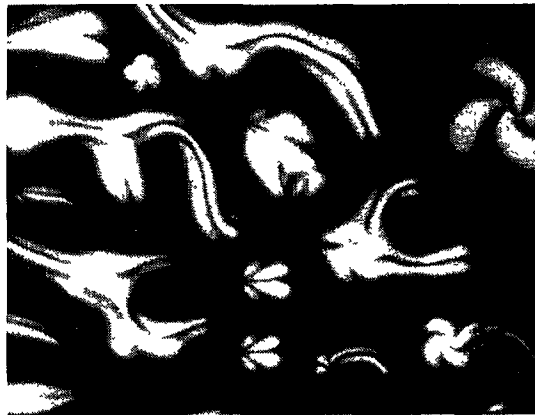
Fig. 7. — Islands transforming into “trefoils” and “spirals” Upper-right corner: a big right-handed spiral with diameter \sim 50 \mu\text{m} . Lower-right corner: right-handed spirals with island-like tails. On their left: two trefoils. Left side of the picture: branched islands. Upper-left corner: a small left-handed spiral. Crossed polarizers parallel to the sides of the picture.
