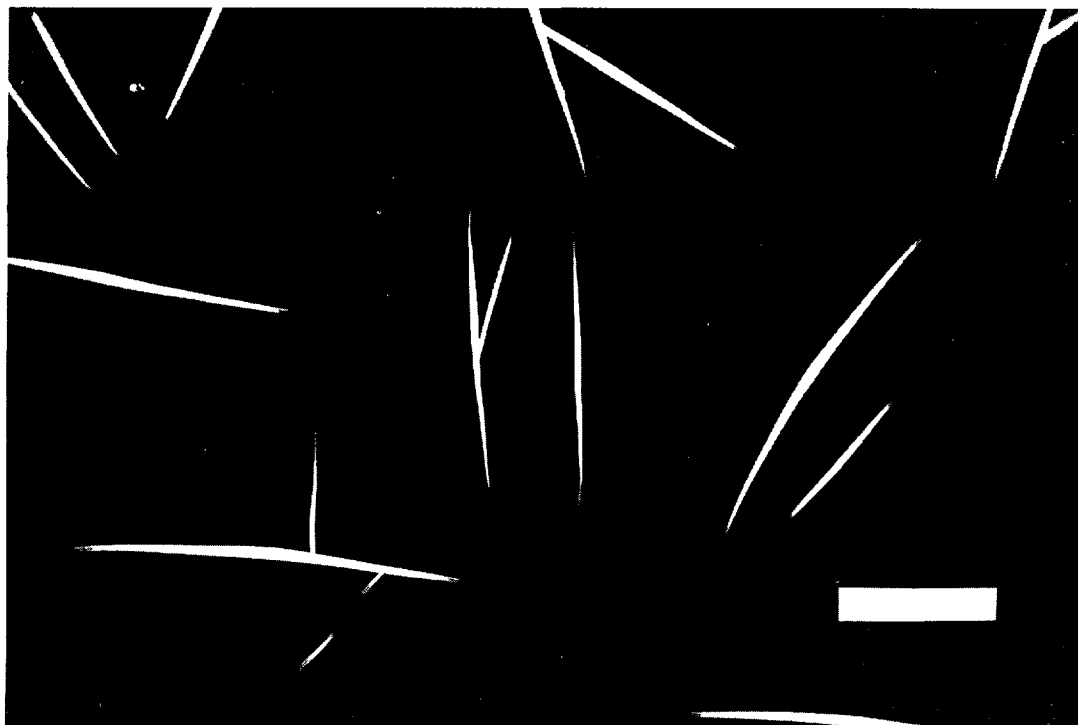
Fig. 2. — Photograph of a NBD-stearic monolayer at the first order solid/liquid phase transition : bright 2D crystals (needles) coexist with the liquid phase. This phase appears to be dark probably because the chains lie on water and the fluorescence of the NBD probes in contact with water is quenched. The bar length is 200 \mu\text{m} .
