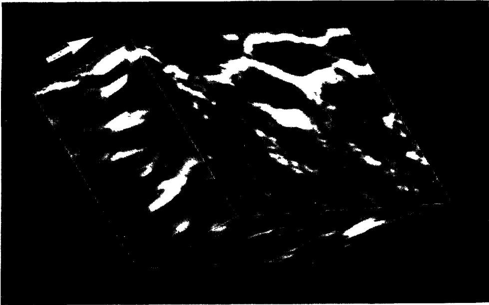
Fig. 6. — Overview of the reconstructed volume (cube of 0.145 \mu\text{m} side) of the 10 % gel from the 2D images seen in figure 5. Once the 3D object is built in the computer memory several procedures can be used for displaying it onto the screen, where the object can be rotated in any direction and observed through several modes : surface, transparent... The arrow shows the direction of the electron beam when the specimen is observed in the untilted position.
