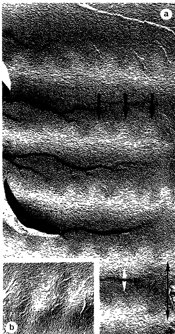
Plate II. — Periodic waves normal to the cholesteric stratification. Molecules parallel or close to the fracture plane draw small periodic waves on one side of each layer (arrows). Note that half of the layer appears undistorted (white arrowheads). The fracture plane is normal to the cholesteric stratification (a, \times 20500 ). Note in (b) the crenelled aspect of these waves, easily visible at higher magnification ( \times 21750 ).
