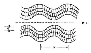
Fig. 10. — Schematic drawing of the undulation instability of the layers in a cylinder of SA.
