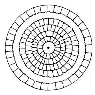
Fig. 5. — A cross-section of the layer arrangement in a spherical S<sub>A</sub> droplet.
