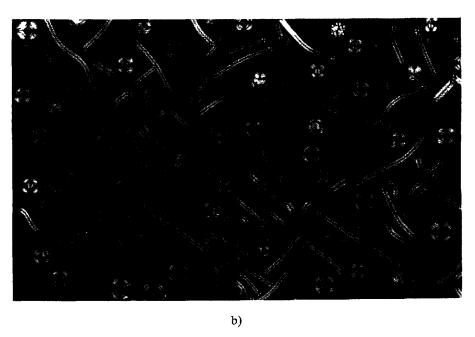
Fig. 7. — a)  $S_A$  cylinders forming in a sample of  $x_{50}$ . Crossed polarisers (× 250). b) Same sample as in figure 7a, photograph taken 10 mn after the cooling was stopped. Note that the cylinders have shrunk in length.
