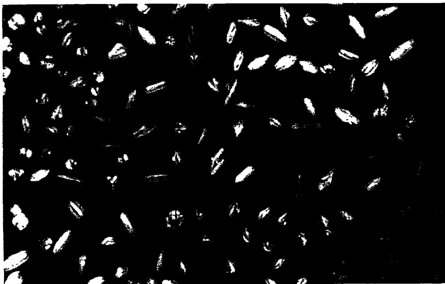
Fig. 2. — The S_A phase separating out from the isotropic phase in the form of batonnets in a sample of diethyl azoxy dicinnamate. Crossed polarisers ( \times 250 ).
