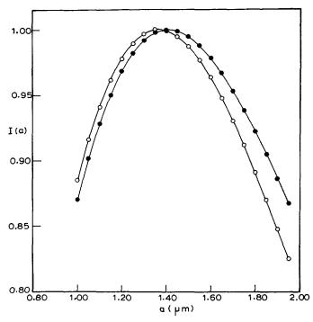
Fig. 14. — Calculated variation of the transmitted intensity as a function of  $\alpha$  a structure, set at 45° between crossed polarisers:  $d\eta/dr = 0.0007$  ( $\odot$ ) and -0.0007 ( $\bullet$ ).
