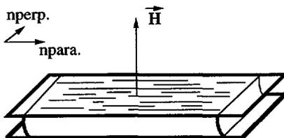
Fig. 12. — Configuration of the samples placed under a magnetic field  $H$ .  $n_{\text{para}}$  and  $n_{\text{perp}}$  are respectively the measured refractive indices parallel and perpendicular to the chain direction.
