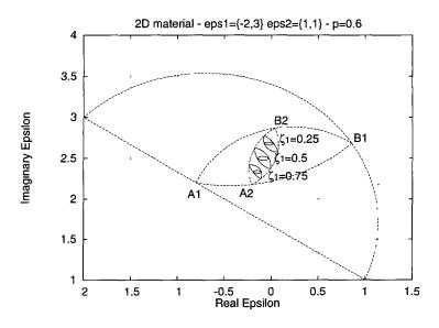
Fig. 2. — Position of the regions  $\Omega^3$  and  $\Omega^4$  (3rd and 4th order bounds) when the function  $\zeta_1$  changes  $(\zeta_1 = 0.25 - 0.5 - 0.75)$ .
