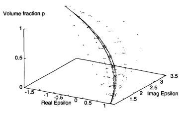
Fig. 17. — Regions  $\Omega^n$  (n = 0, ..., 4) of the complex plane filled by the values of  $\epsilon_e$  when p varies.
