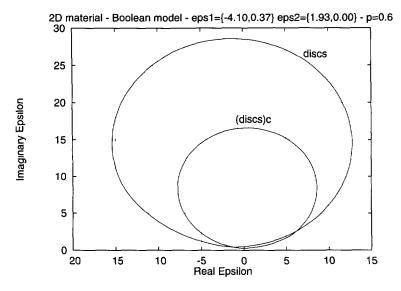
Fig. 5. — 4th order bounds  $\Omega^4$  for Boolean models of discs and  $(\text{discs})^c$ . Example where  $\epsilon'_1 \epsilon'_2 + \epsilon''_1 \epsilon''_2 < 0$ : the regions are overlapping.
