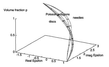
Fig. 20. — 4th order bounds for mosaic models of discs, Poisson polygons, and needles.
