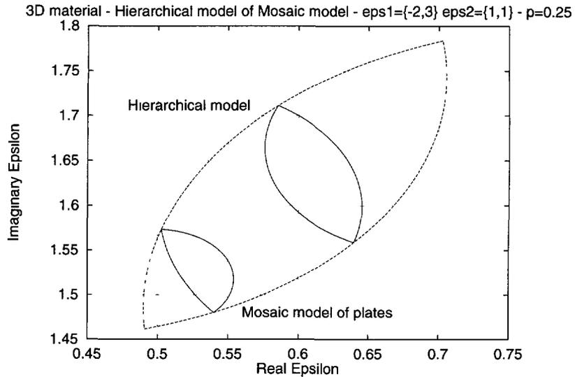
Fig. 26. — Bounds for a hierarchical model of mosaic with plate cells (2nd and 3rd orders).
