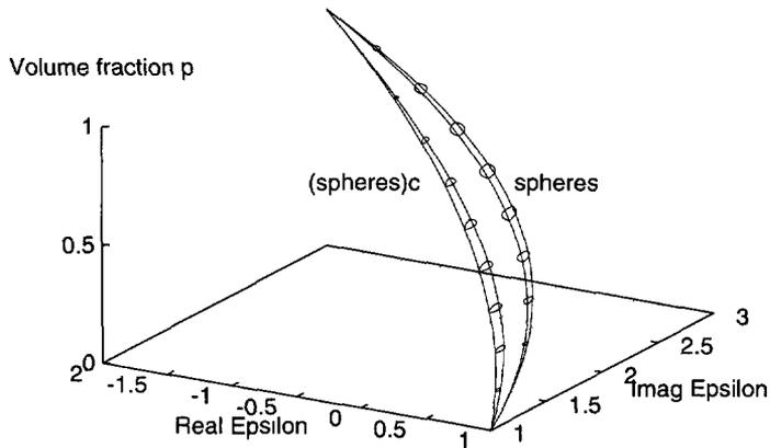
Fig. 24. — 3rd order bounds for the Boolean model of spheres and  $(\text{spheres})^c$ .
