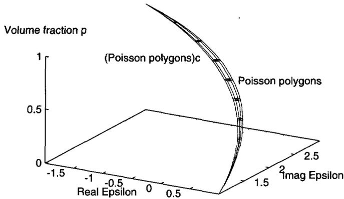
Fig. 19. — 4th order bounds for the Boolean model of Poisson polygons and (Poisson polygons)<sup>c</sup>.
